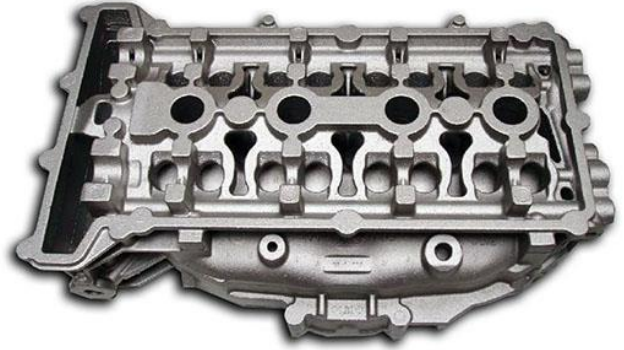
Complex engine casting with feeders removed
