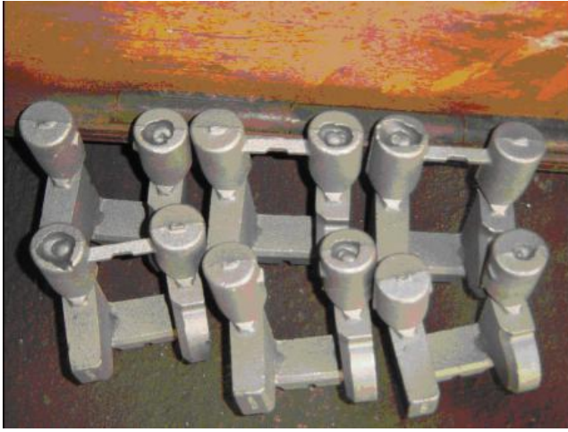
Simple castings with feeders attached
